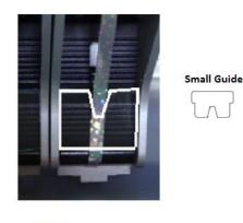
Small Guide is inserted in the front with Slot facing Upwards.
